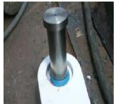
The ThorPlas-Blue SAB and hard coating pin system can be ordered in 4 standard pin sizes of 1.5", 2", 2.5" and 3", as well as in custom sizes.
